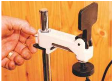
▲ This quick-release clamp is very fast to adjust
